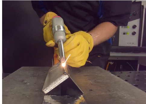
Fixtureless Joining of Materials with Dissimilar Thicknesses
