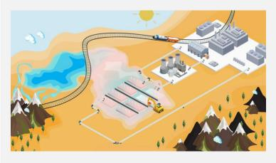
Our operation utilizes solar and wind evaporation over a three-year pond process developed to access minerals
