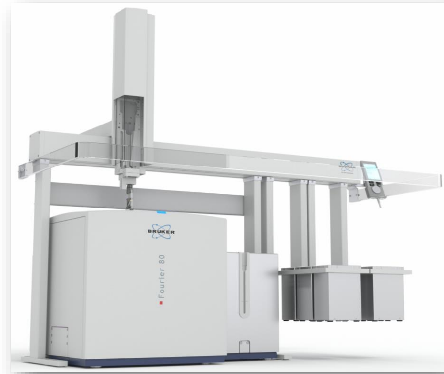
Gradient-spectroscopy Fourier 80 with PAL sample changer
