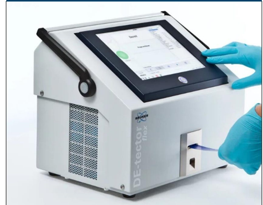
DE-tector Flex: explosives trace detection for air cargo, and Europe/Middle East passenger screening
