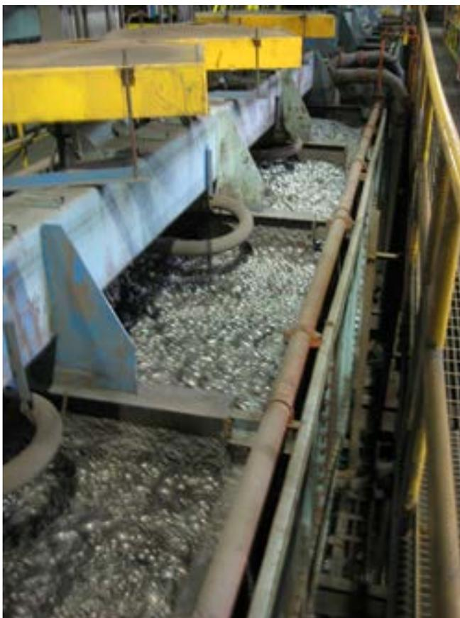
**Figure 2:** Caribou mill zinc flotation circuit. Concentrate is being stockpiled in the onsite warehouse.
