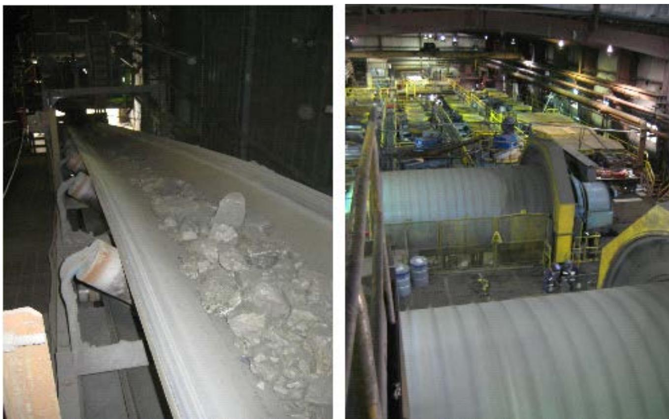
**Figure 1:** Crushed UG feed being conveyed into the SAG Mill for finer grinding (left). Ball Mills in foreground with flotation circuits in background at Caribou Mill (right).
