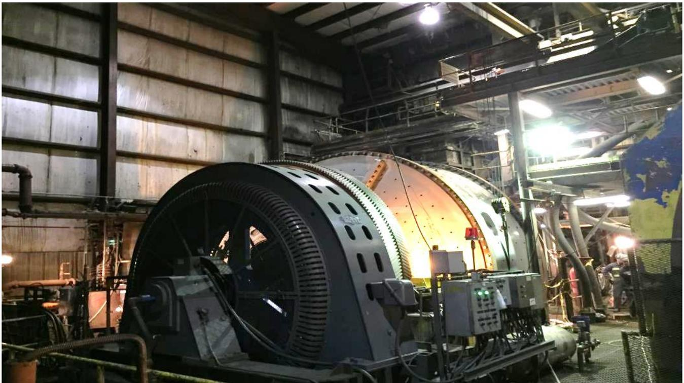
**Figure 1: Newly installed 3,000-tpd SAG mill at Caribou**
