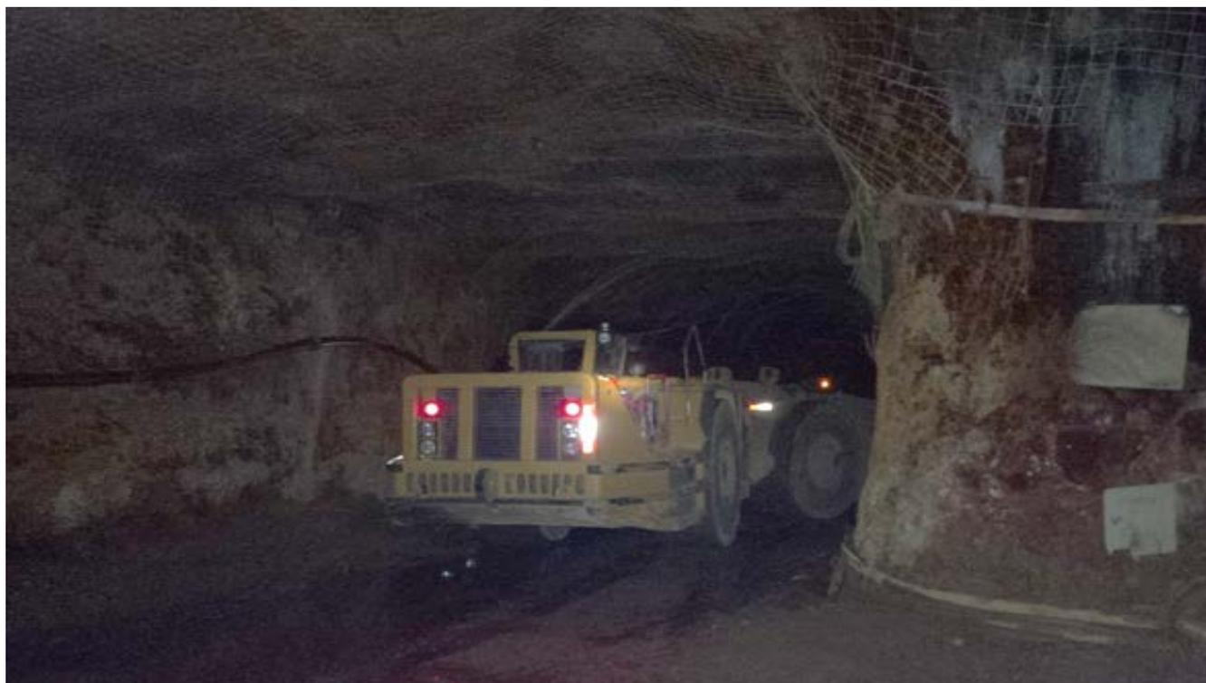
**Figure 3: Scoop tram operating underground at Caribou.**
