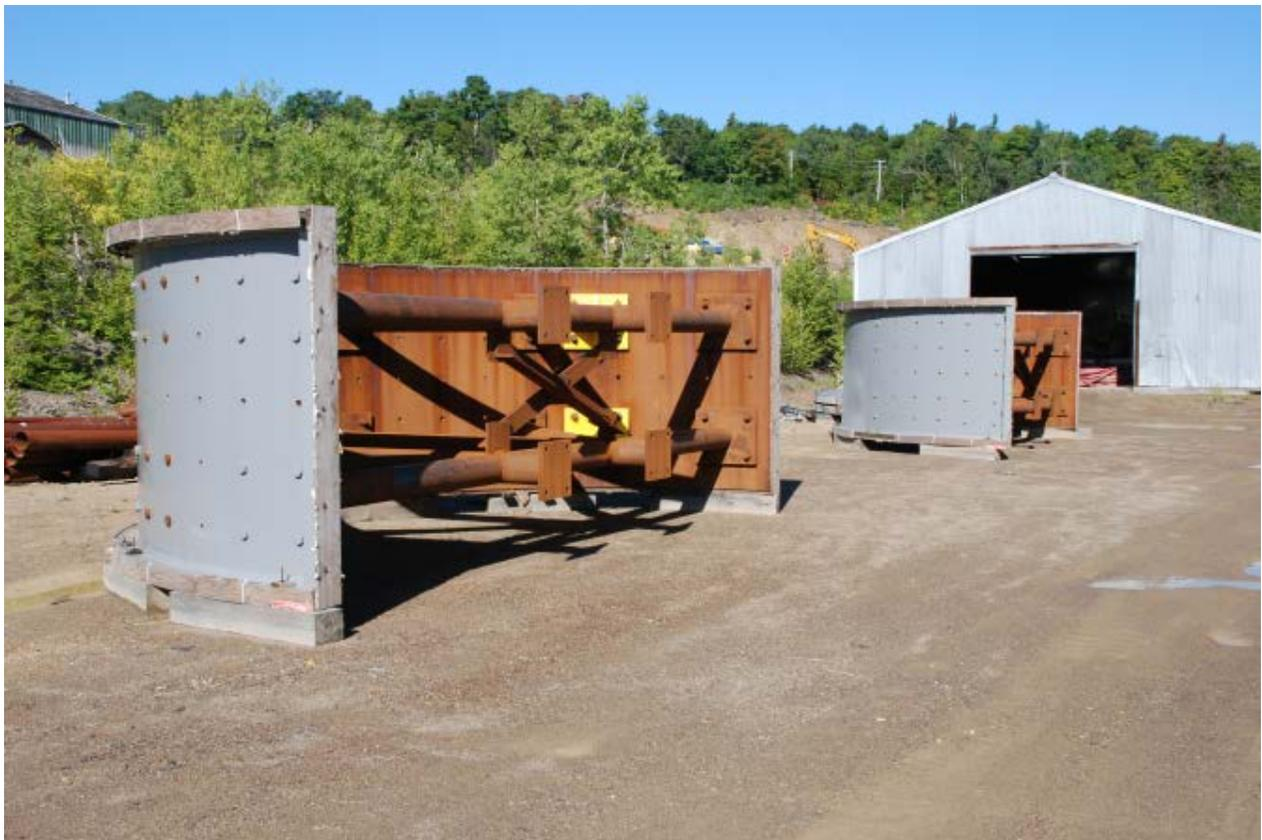
**Figure 2: New 3,000-tpd SAG mill and components are onsite for installation in the Caribou Mill**
