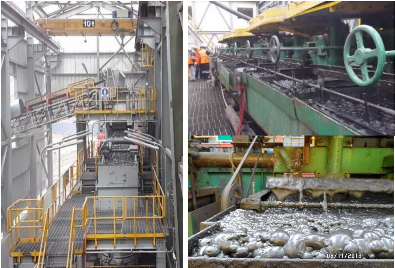
**Figure 1:** Crushing circuit (left) and zinc scavengers and flotation circuit (right).
