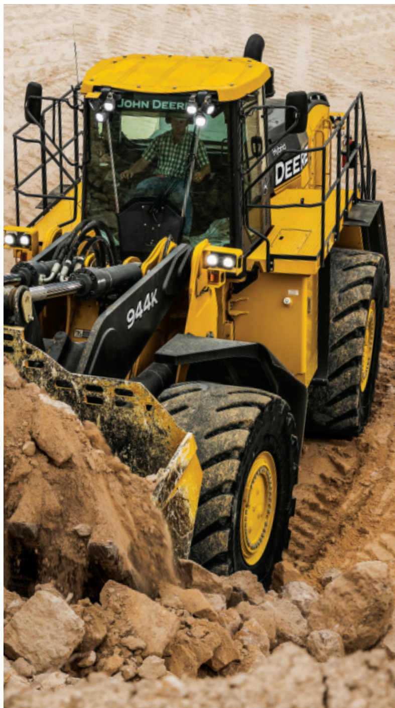
The 944K hybrid wheel loader advances Deere's lineup of production-class machines. Its 536-horsepower engine with hybrid-electric drive differentiates the 944K, helping deliver up to 40 percent fuel savings compared with conventional drivetrains.
