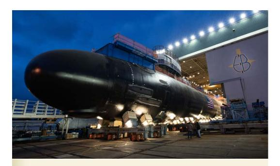
Electric Boat participates in the U.S. Navy's SUBSAFE program, which establishes an extremely high level of quality assurance for components used in nuclear-powered submarines. SUBSAFE has rigorous controls on systems that are essential to water-tight integrity, requiring that parts have traceable evidence of quality from the point of manufacture to the point of installation, including records of the creation of the product and its source materials.
