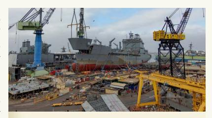
NASSCO has reduced its reliance on diesel equipment to decrease its emissions. The shipyard has more than 90 electric cranes and uses exhausted treatment systems and filters for equipment with large diesel engines. Since 2004, NASSCO has reduced overall diesel emissions by 80%. In 2022, NASSCO introduced a pilot program to use renewable diesel fuel in the shipyard that lowers particulates by 30% and reduces greenhouse gas emissions by more than 80% compared to traditional diesel fuel.
