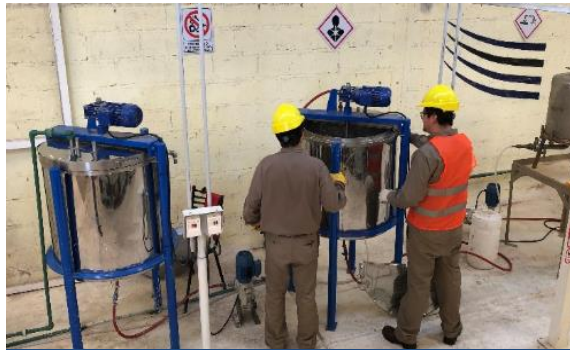
2: Sulfatation for Ca Removal
